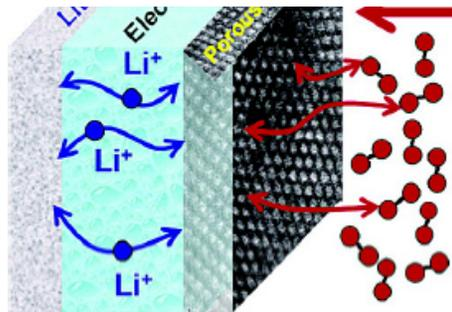
Polymer gel and polymer hybrid membrane based ionic electrolytes for Li-air batteries (collaborated with Jim Zheng @ EE)
